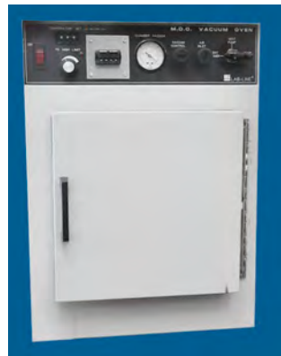
Figure 1. Ideal vacuum oven with metal door. Glass doors are heat sinks and contribute to variable results in moisture tests.
